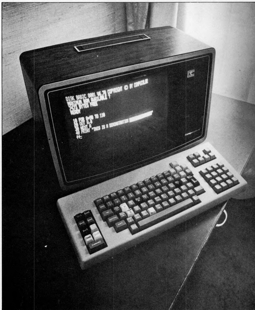
The Compucolor II — disc drive, colour video and pitched at Apple prices.
